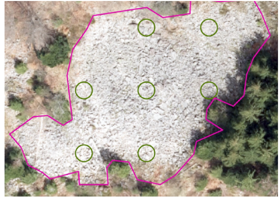
Fig. 2: Aerial photo with block field margins and subplots used for representative counts of stone density. Subplots have a 2 m radius.
